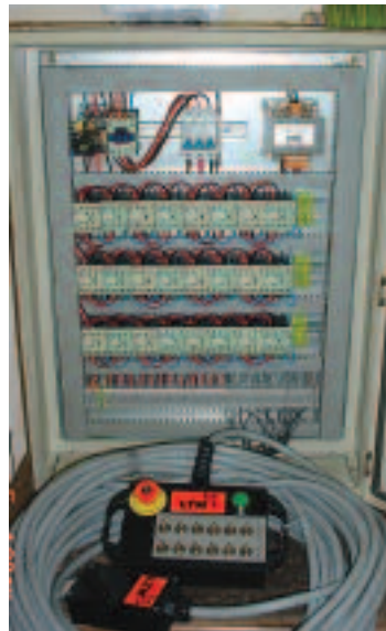
Wall mounted controller 12 Channel direct control - hardwired
