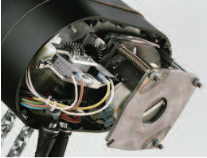
New mechanical components and electrical wiring at brake end of lodestar
